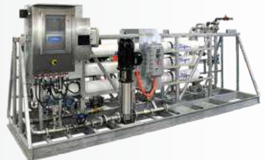
Culligan® built this RO to meet a client's rigid refinery specifications, including galvanized skid, B31.3 piping, Class 1 Div. 2 Explosion Proof controls, high temperature operation at 130°F, duplex cartridge filters and duplex feed pumps with Allen Bradley PLC and HMI.
