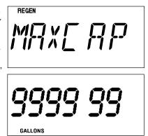
• Batch Set Point - This setting is used to set the trip point for regeneration when in flow meter operation. It will only appear if a flow meter is connected. The programmed setting displays the actual set point to trigger regeneration. The display will show the "REGEN" icon and "bAtch" for two seconds and then display the "REGEN" and "GALLONS" or "LITERS" (depending on dip #7 setting) icons and the setting numbers to adjust. Adjust the value with the "Up" or "Down" keys.
